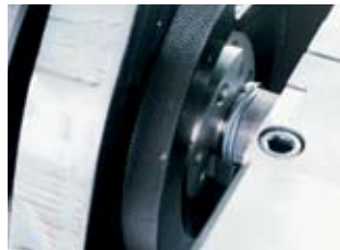
REMOVAL OF FRICTION WELDING FLASH BY STAMPING
