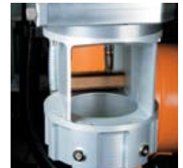
Cross jet / cone jet function for the avoidance of nugget fouling and plasma in the weld pool
