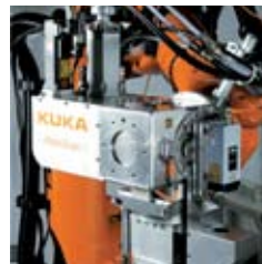
Plug & Play distance sensor for direct transfer of distance information to the robot program
