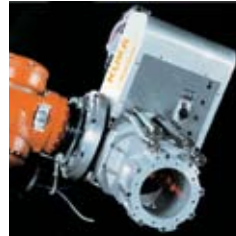
Simple teaching with two integrated program pointers which cross at the focus
